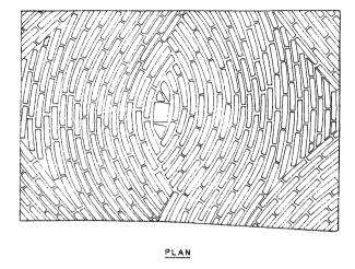
Figure 7 Plan and section of pitched-brick vault on pendentives, Tell al Rimah, late third millennium BC.
