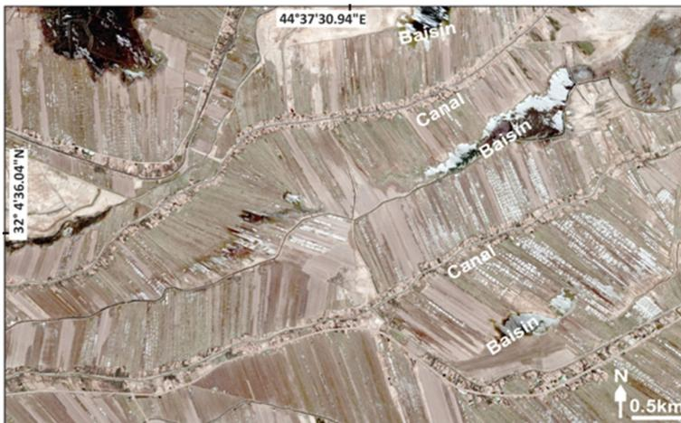
**Fig. 4** Herringbone pattern of fields in the western plains showing the canals on raised ground and the basin soils between. Note occasional areas of salinization around some basin areas (by Jaafar Jotheri)
